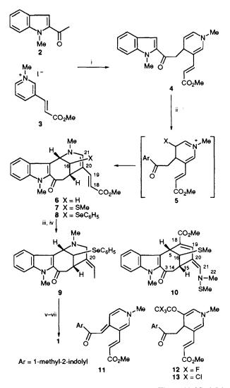
Scheme 1 Reagents and conditions: i, LDA-THF, -30 °C, 1.5 h; ii, DMTSF or C<sub>6</sub>H<sub>5</sub>SeBr, -30 to 0 °C, 3 h; iii, 4 mol dm<sup>-3</sup> HCl, 100 °C, 2 h; iv, NaBH<sub>4</sub>, MeOH, 0 °C, 1 h; v, MCPBA, CH<sub>2</sub>Cl<sub>2</sub>, -70 °C, 20 min; vi, LDA, ICH<sub>3</sub>, THF, -70 °C, 1 h; vii, diisopropylamine, THF, reflux, 1 h
